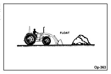
Float will also prevent mixing of surface material with stockpile material. Float position will reduce the chance of surface gouging when removing snow or other material.
